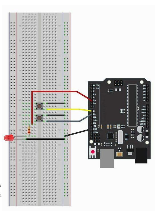
Although the bodies of the switches are square, the pins protrude from opposite sides of the switch. This means that the pins will only be far enough apart when they are placed correctly on the breadboard.
