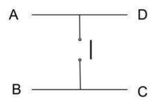
Actually, there are only really two electrical connections. Inside the switch package, pins B and C are connected together, as are A and D.
